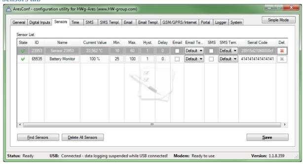
Use this tab to configure basic and advanced properties of sensors:
