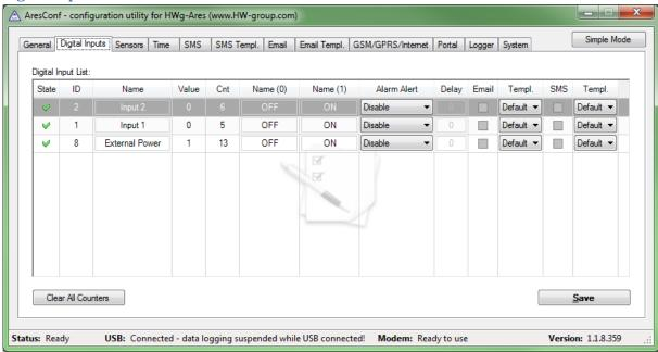
Use this tab to configure basic and advanced properties of digital inputs:
