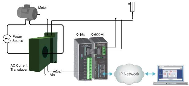
This example uses a current sensor that will measure current up to 20 Amps AC. The sensor produces a linear 0-5VDC output that it can be connected directly to one input of the X-16s analog module. The slope is calculated and entered into the setup pages of the X-600M. The slope calculation is given below:
