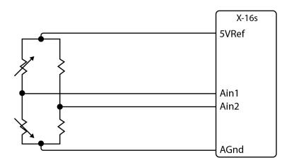
The low input bias and high resolution inputs of the X-16s together with the reference output make the X-16s workable with many bridge sensors without using a preamplifier or other circuitry.
