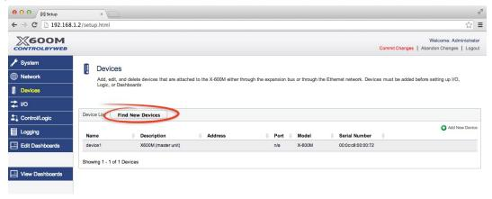
2. In this example we are going to add an *X-13s Thermocouple expansion module*. Click the **Add** button for the X-13s.
