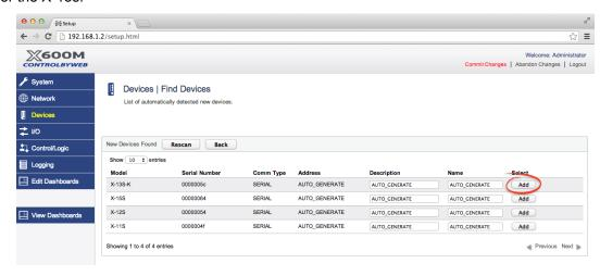
3. In the *Select* column, click the checkboxes of the I/O components you would like to configure and select the **Create Device Widget** checkbox (This will display the status of the I/O on the Dashboard).
