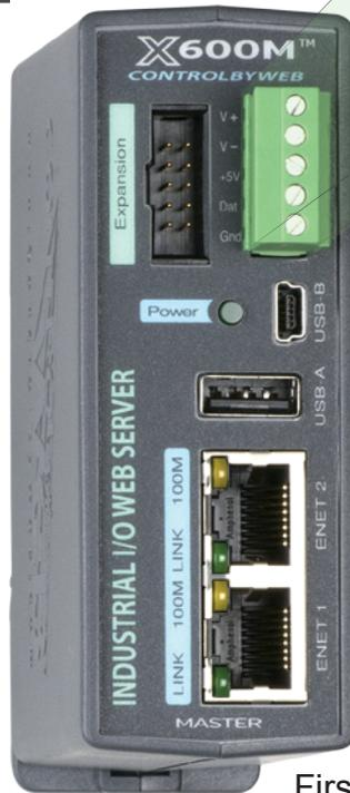
**Warning:** The maximum number of attached expansion modules is determined by power supply voltage, power supply current, and type of modules attached. For some installations, additional power supplies and expansion bus power injectors may be required.
