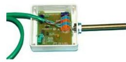
To connect sensor that is not at the end (so it's MIDDLE) you must connect the green and the blue wire of the TP cable on the sensor's connector - as you can see on the picture. Be careful, you always connect full colour with striped colour.
