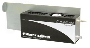
Module (PSM) may also be added for power redundancy. If the first PSM fails, the second PSM will take over the entire load and carry on normally. Additionally, if one PSM fails, an onboard alarm will sound. An LED indicates that the +9VDC output voltage is present, and that the module is operating properly.
