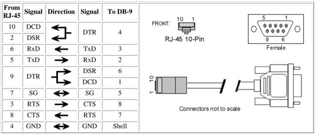
\* Arrows indicate which direction the signal is flowing
