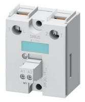
Semiconductor relay, 1-phase 3RF2 Overall width 45 mm, 50 A 48-460 V / 4-30 V DC screw terminal
