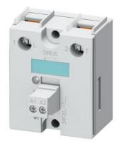
Semiconductor relay, 1-phase 3RF2 Overall width 45 mm, 50 A 48-460 V / 24 V DC screw terminal
