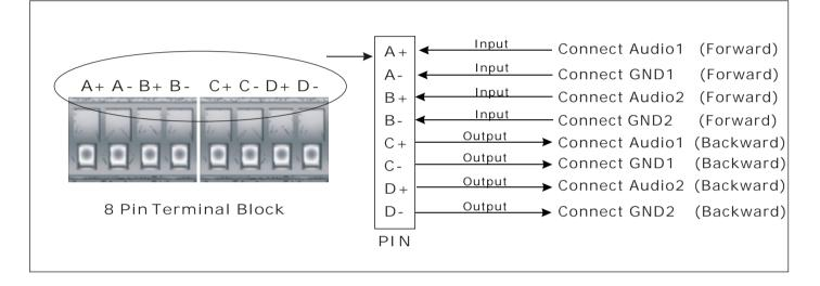
Receiver (Audio): 2-Channel Duplex Audio Connection (Input/Output)
