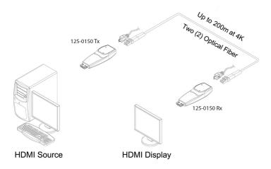
Figure 1 - Overall Connection of 125-0150
