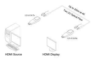
Fig Figure 4 - Connection with optical fiber
