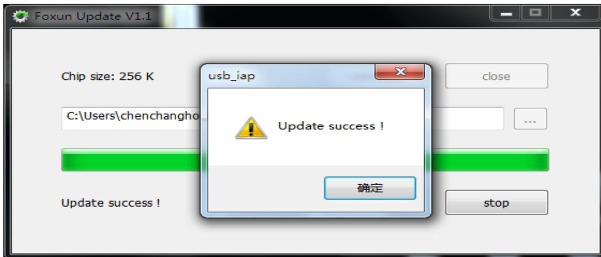
Note: If the connection is upgraded to half current, the upgrade progress bar will stop. At this time, the device should be powered off and restarted before USB upgrade.
