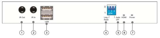
(1) **IR Out:** Connect to the supplied IR blaster cable for IR signal transmission. Place the IR blaster in direct line of sight of the equipment to be controlled.
