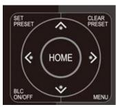
**Set Preset:** Press the [SET PRESET] button, then press the number buttons 0-9 to set the preset positions.
