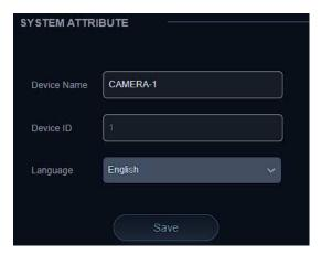
**System Attribute** allows users to edit the Device Name of the camera which can be helpful when identifying devices through enterprise level networks.
