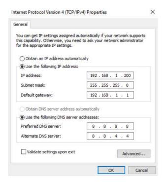
**NOTE:** When you are finished configuring the camera you will need to return to this screen and select 'Obtain an IP address automatically' and 'Obtain DNS server automatically' to restore internet connectivity to your computer. Also make sure to reconnect any ethernet cables you may have unplugged.
