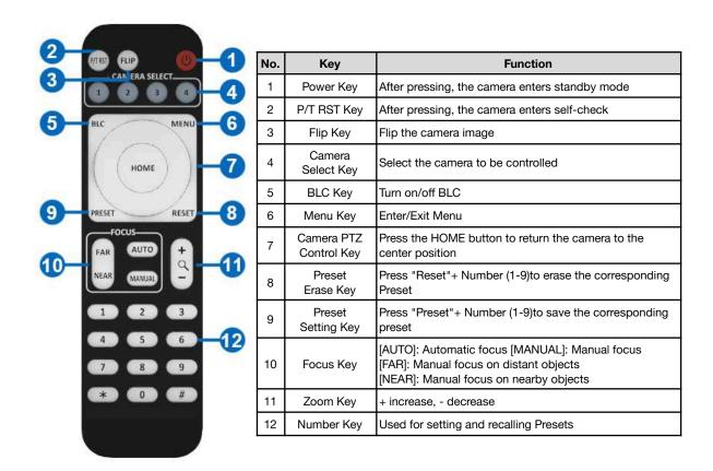
**Note:** Always maintain a direct and unobstructed line of sight between the remote control and the sensor on the front of the camera.
