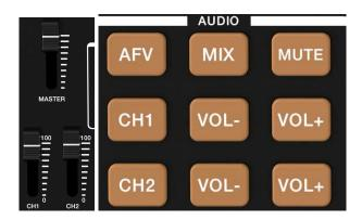
The BG-QuadFusion-4K supports analog balanced audio input and output, HDMI audio extraction, as well as audio matrixing using the Audio Follow Video (AFV) and MIX functions.
