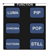
LUMA: Removes the color black from the background of the PVW image and overlays the remaining imager on top of the PGM output. Typically used to place a watermark, logo, text, or subtitles on the PGM output
