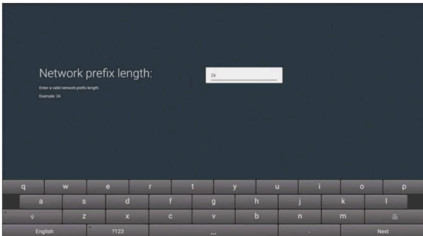
Network prefix length sets the network subnet mask. A setting of 24 is equivalent to setting the mask to 255.255.255.0
