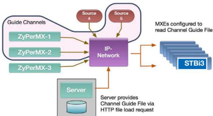
In the diagram shown, if the guide file is specified as exclusive, and the only entries in that guide file are for ZyPerMX-1, ZyPerMX-2, and Source 5, then any other channel will be ignored and not included in the guide. The only stream the user will be able to select are for the channels described in the guide file.
