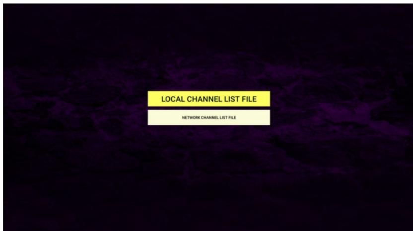
In the dialog, enter the pointer to the location on the web server where you have placed the Channel Guide file. Local Channel List File would be located on a USB memory stick plugged into one of the STBi3 USB ports. The location of a Network Channel List file depends on where the IT admin has allowed HTTP file browsing to.
