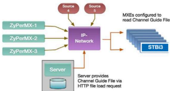
If the guide file is in “Additive” mode only the non-ZeeVee channels need to be specified in the guide file. The ZeeVee channels will send beacons that are learned by the STBi3 and those channels will automatically be added to the guide. In the diagram shown Source4 and Source5 are streams supplied by non-ZeeVee equipment. Only stream information for Source 4, and Source 5 need to be specified in the guide file.
