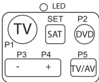
The upper-left portion of the remote houses a set of programmable keys. The intent is to allow for common television functions to be programmed so the user only needs to use a single remote control device to manage their television experience when using the STBi3 receiver/decoder.
