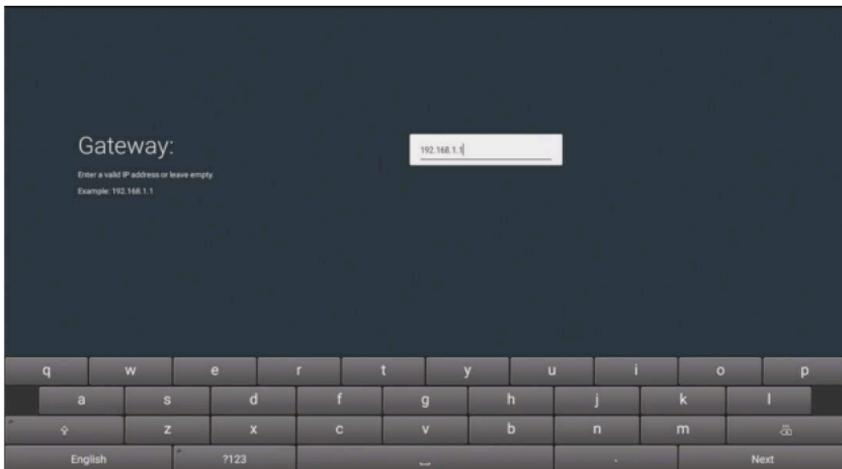
Once the IP address, Mask, Gateway and DNS are entered manually, highlight "Submit" and click the OK button on the remote.
