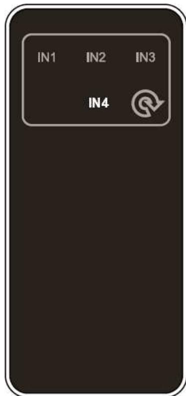
**IN1/2/3/4 :** Press the IN1/2/3/4 button to select the desired HDMI signal source for the OUTPUT port.
