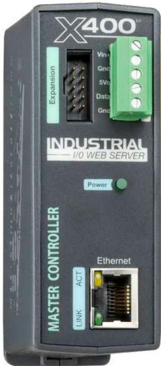
The X-400™ is a powerful web-enabled industrial I/O controller with advanced logic and modular expansion capabilities.
