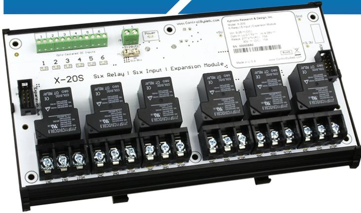
The X-20s™ expansion module is used with the X-600M controller. The X-20s has six, high-current relays, each with Form-C contacts (SPDT) and six, optically-isolated digital inputs. A screw terminal strip provides high-current connections to the relays.
