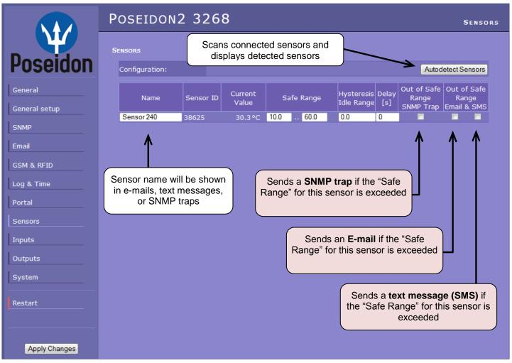
After connecting sensors or changing RJ11 connections, sensors need to be detected again.
