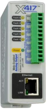
The X-417™ is a web-enabled analog output module with five output channels. The analog outputs are similar to that of a Programmable Logic Controller (PLC). However, unlike a PLC, the X-417 is designed for web-based applications from the ground up. No add-on software or hardware is required.
