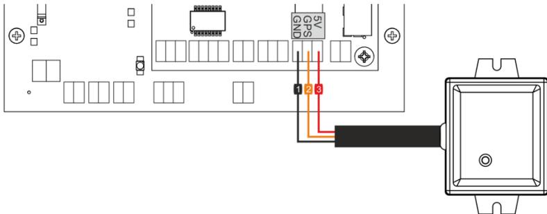
fig. 7 Connection the GPS module to the clock
