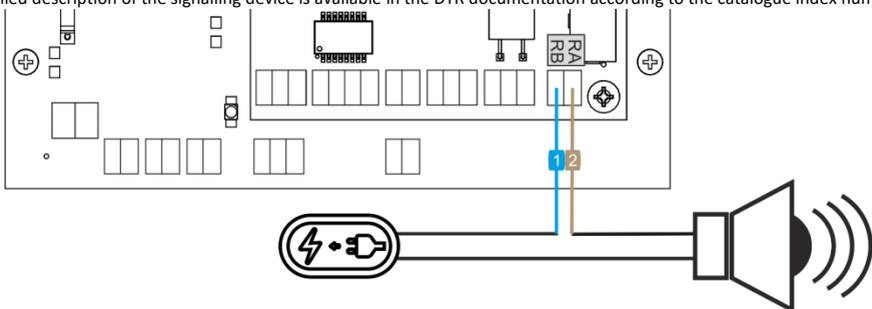
fig. 9 Buzzer and clock wiring diagram
