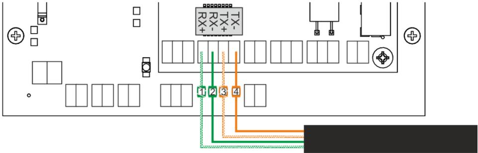
Fig. 4 LAN and clock wiring diagram
