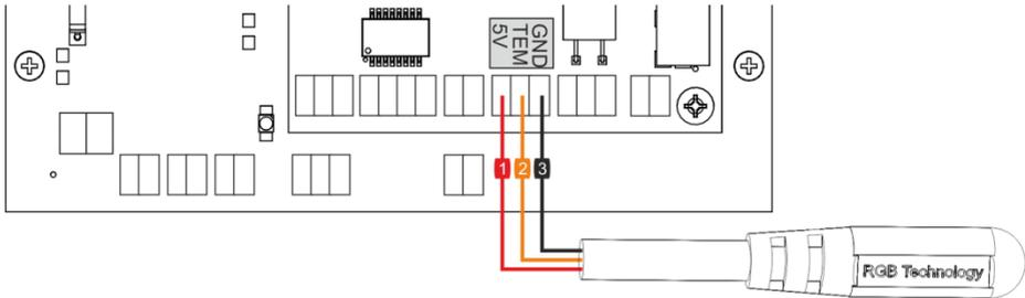
fig. 8 Temperature probe and clock wiring diagram
