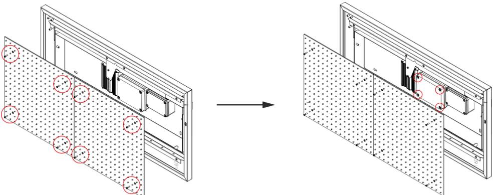
fig. 2 Disassembly of diode modules and housing cover
