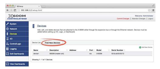
2. In this example we are going to add an *X-11s* | 2 Relay expansion module. Click the **Add** button for the X-11s.
