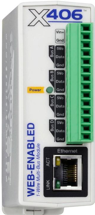
The X-406™ is a fully-featured, web-enabled temperature and humidity module with four independent 1-Wire Buses that allow for monitoring up to 16 temp/humidity sensor per bus, for a total of up to 64 sensors.
