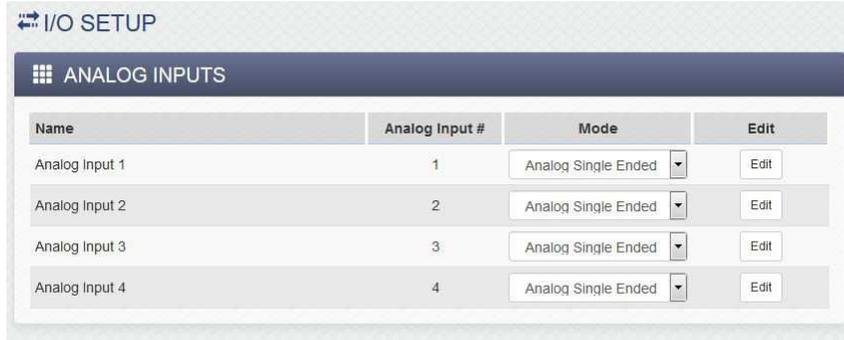
The X-420 features a high performance, 4-channel, 16-bit analog data acquisition system. Each analog input can be configured separately:
