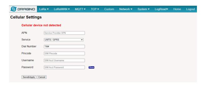
Note \*: For DLOS8N which doesn't have the cellular module, this page will shows Cellular not detected.
