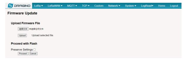
Select the required image and click **Flash Image**. The image will be uploaded to the device, and then click **Process Update** to upgrade.
