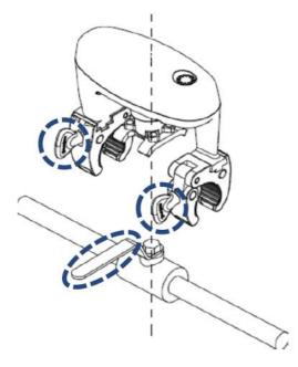
Installation Step 3: Align the fork with the valve handler
