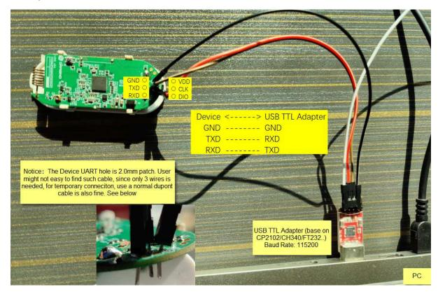
In PC, User needs to set **serial tool**(such as <u>putty</u>, SecureCRT) baud rate to **115200** to access to access serial console of LWL02. Below is the output for reference:
