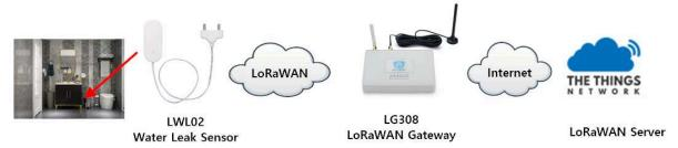
The LWL02 has water leak detect probe as above. When there is water between these two detect probe, they will be short and generate the water leak event. and send the status to LoRaWAN server. The LWL02 will uplink two type of messages to the server.
