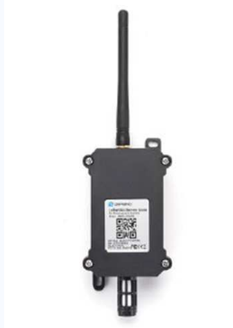
On device SHT31 Probe
