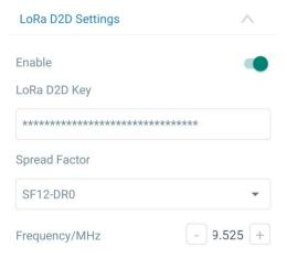
3. Enable one of WS301 status and configure a 2-byte hexadecimal command (This command is pre-defined in LoRa D2D agent device). When WS301 detects this status, it will send the control command to corresponding LoRa D2D agent devices.
