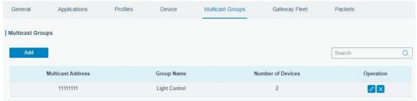
3. Go to **Network Server > Packets**, select the multicast group and fill in the downlink command, click **Send**. The network server will broadcast the command to devices which belongs to this multicast group.
