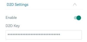
4. Enable one of WS101 button mode and configure a 2-byte hexadecimal command (This command is pre-defined in Milesight D2D agent device). When you press as this button mode, WS101 will send the control command to corresponding Milesight D2D agent devices.
