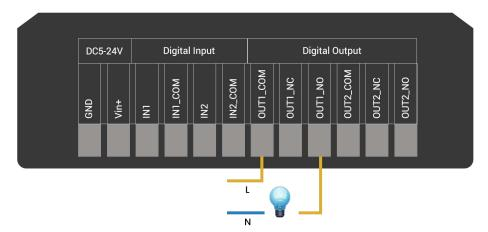
• When the output is off, the COM and N/C terminals will be internally connected to each other. Here is a schematic of the output circuit:
