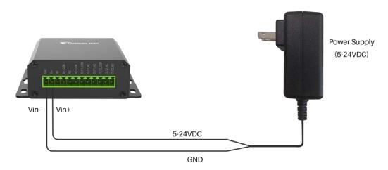
For industrial applications, it is advised that the Ursalink UC1114 should be installed into its own metal housing and be powered from a separate power supply (as opposed to sharing one with other equipment).
