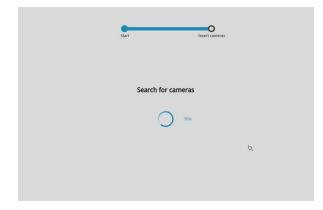
4. All cameras detected on the network will be automatically listed. If necessary, deselect the cameras you want to exclude from the configuration.
