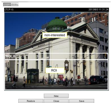
As the result, the lower screen is constantly displayed in high details, while the upper half is transmitted using a lower-quality format. Although the upper half is transmitted using a lower quality format, you still have an awareness of what is happening on the whole screen.
