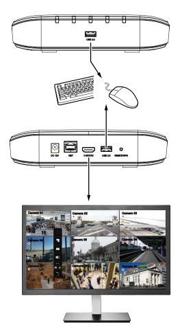
By default, a live view appears on an HDMI monitor. The interface architecture of the local console is illustrated as follows:
