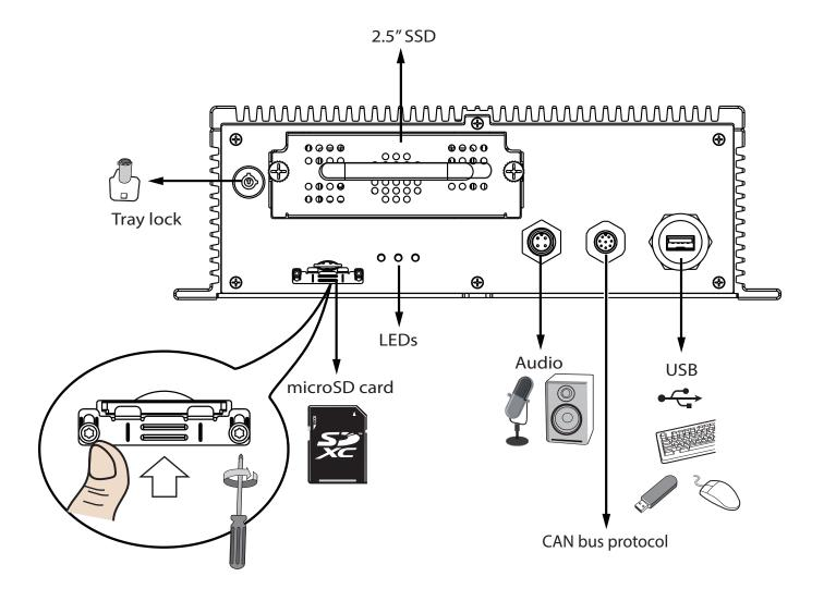
You should pull the retention cap up after you install an SD card to prevent disconnection by vibration or impact.
