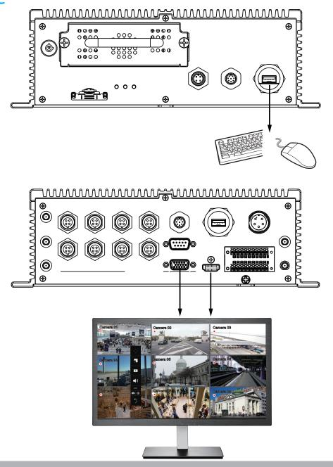
By default, a live view appears on an HDMI monitor. The interface architecture of the local console is illustrated as follows:
