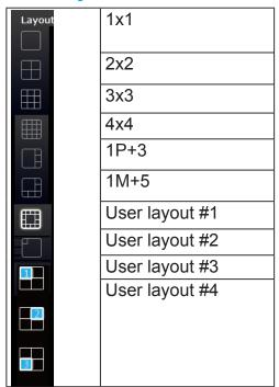
By default, 5 typical layouts are provided for the user. They include: 1x1, 2x2, 3x3, 4x4, 1P+3, 1M+5, and 1M+12. System default is the 4x4 layout. Cameras that do not fit into the first page of a layout, say, a 3x3 layout, will be displayed on the succeeding layout pages.
