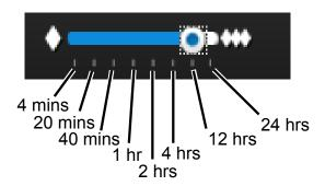
You can use the timeline zoomer to scale down the span of time. For example, if the time span is reduced to 1 hour, then each section on the time line represents 15 minutes of recording. The total time span on a timeline starts from the minimal of 4 minutes, 20 minutes, 40 minutes, 1 hour, and up to a maximum of 24 hours.
