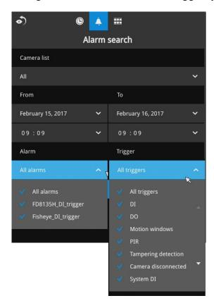
When done with the selection, click on the Search button. In the sample screen below, a list of alarms is displayed, and you can click on any of them to replay the moment when the alarm was triggered. The alarm-related recording will typically include a length of 5 seconds of pre-alarm and 20 seconds of post-alarm footage.
