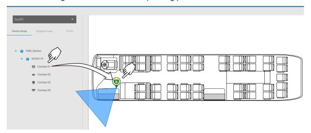
When the camera is in place, drag the FOV indicators on the edge to change the shoot angle and the coverage range.
