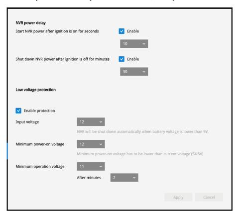
The low voltage protection feaure enables the system to be powered down after the low voltage condition persists for a configurable period of time.
