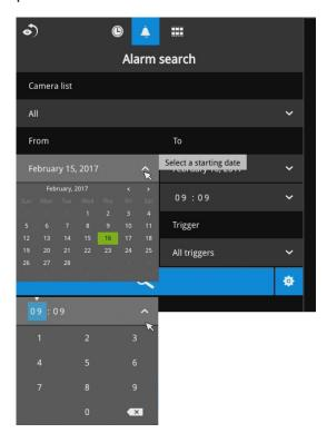
You can also determine what types of alarms will be included in the search. Select the preconfigured Alarms or select the Trigger types from the pull-down menus.
