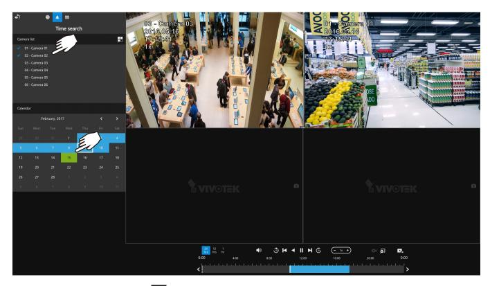
Use the layout button to adjust view cell arangement on screen. You can retrieve the recorded videos from a max. of 4 cameras at the same time.
