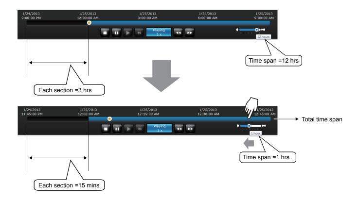
If recordings take place by an event-triggered recording, the intervals between recordings can be down to 1 minute, and the individual recordings will not be easily discernible. In this situation, you can mouse over the timeline to pinpoint individual recording instances.
