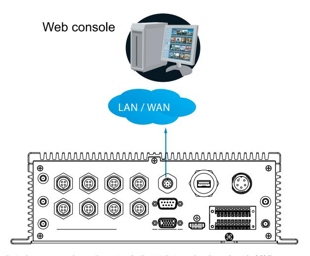
Note that when accessed over the network, the total streaming throughput is 96Mbps.
