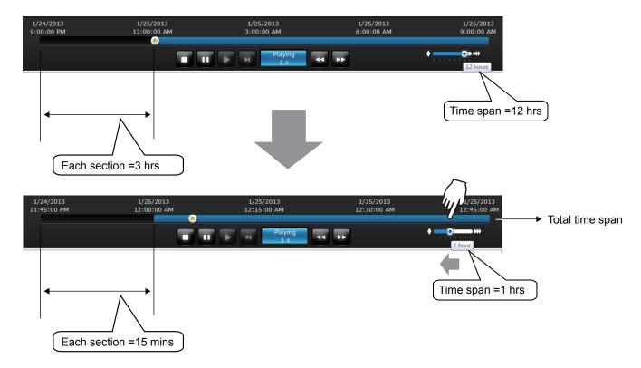
If recordings take place by an event-triggered recording, the intervals between recordings can be down to 1 minute, and the individual recordings will not be easily discernible. In this situation, you can mouse over the timeline to pin-point individual recording instances.
