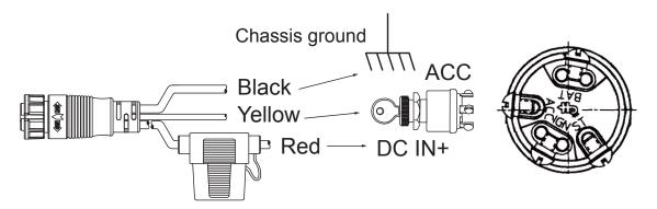
Connect the yellow wire to a vehicle's ignition switch's ACC pin. Red wire to the vehicle battery output, and the Black wire to the chassis ground.
