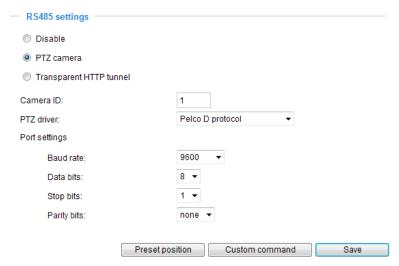
VIVOTEK provides the following PTZ drivers: DynaDome/SmartDOME, Lilin PIH-7x00, Pelco D, and Pelco P protocol. If none of the above PTZ drivers is supported by your PTZ scanner, please select **Custom camera** (scanner). Please refer to the documentation of your PTZ scanner to determine the Camera ID, PTZ driver, and Port settings. The Camera ID is necessary to control multiple cameras. If you click **Save** to enable this function, the camera control panel will be displayed on the main page.
