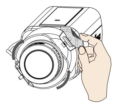
Fasten the lens module to the camera, and notice that the lens module does not block the the light sensor. You can still turn the camera when the lens module is secured to the camera .
