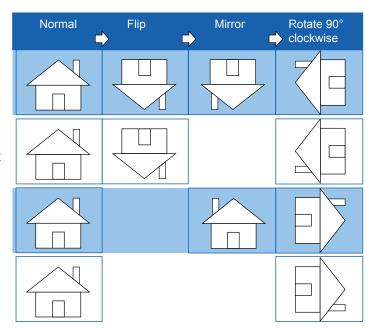
The camera may be installed on a vertical, side-facing, or tilted surface in order to accommodate the interior or exterior design of a building. The interior of a building can be shaped as a narrow rectangular space, such as corridor. The conventional HD image, such as that of a 16:9 aspect ratio, will be incongruous with its wide horizontal view. With video rotation, the camera can more readily cover the field of view on a tall and narrow scene.
