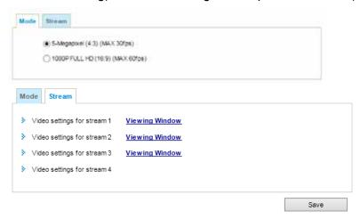
This Network Camera supports multiple streams with frame sizes ranging from 320 x 240 to 2560 x 1920 pixels.
