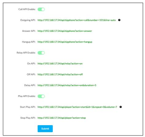
(Note: Authentication and encryption are not used in the API interface, so please pay attention the security of the network environment when opening and using these API interfaces).
