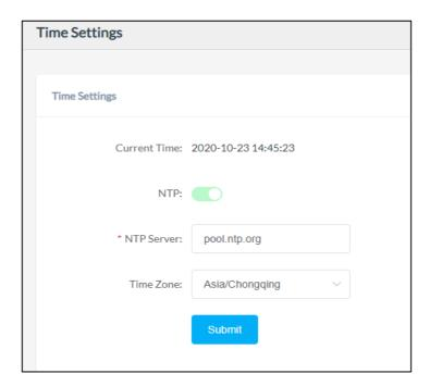
Here you can change a NTP server by modify the NTP server address and you can select the time zone of your location, so the network speaker will synchronize time of your time zone from the NTP server you have configured.
