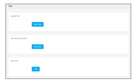
Speaker Detection: Click on the Start button, the speaker will play a ringtone to test whether the speaker is working.
