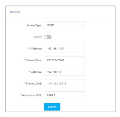
Turn the DHCP switch button off to show the network parameter settings.
