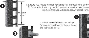
Insert the Rackstuds<sup>™</sup> sideways (spring section towards the centre of the rack) and at 45°.
