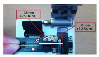
5) Cut the bare fiber of 125um to be 8mm with a cleaver
