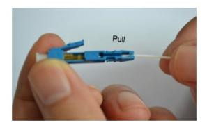
10) Keeping the fiber straight, pull the tight buffer (900um) back
