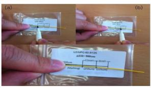
2). Mark on the tight buffer (900um) with (a), (b) for strip
