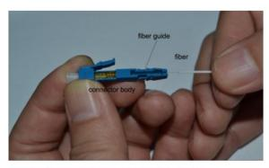
7) Insert fiber in the connector body through the fiber guide
