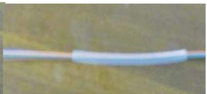
Pic5: use EVA tube to protect stripped fiber
