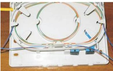
Pic14: after shrink, splice protective tube put into the slot of tray
