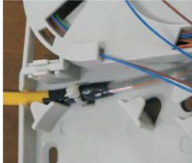
Pic12: put the pigtail through into the
