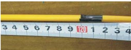
Pic3: the length of stripped fiber cable
