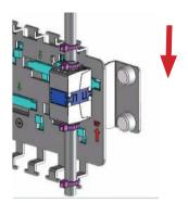
Secure the coupler housing and shield contact via cable tie. Fix the cable to the strain relief via cable tie.
