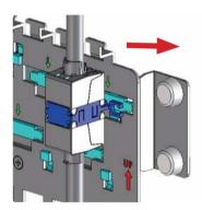
Put the coupler in the provided opening. Slide it down until the plastic latch locks.
