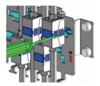
Push the plastic latch with a screwdriver to inside and slide the coupler on the corresponding side upwards.
