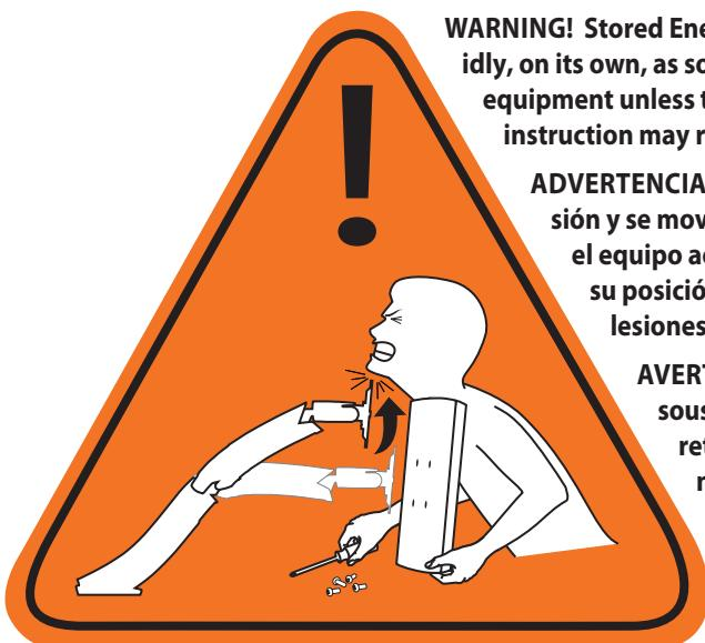
**WARNING! Stored Energy Hazard:** The arm mechanism is under tension and will move up rapidly, on its own, as soon as attached equipment is removed. For this reason, DO NOT remove equipment unless the arm has been moved to the highest position! Failure to follow this instruction may result in serious personal injury and/or equipment damage!
