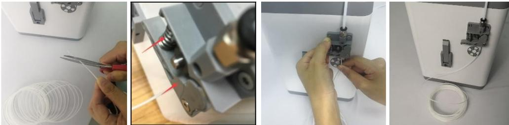
4. Press the Knob to start loading filament. Once filament starts extruding from the Nozzle, press the Knob again to stop extrusion. Clean the extruded filament, then press the Knob to select the Continue option.
