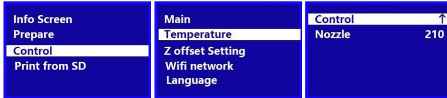
1. On the Main Menu, rotate the Knob until the Control option is highlighted, then press the Knob to enter the Control Menu.
