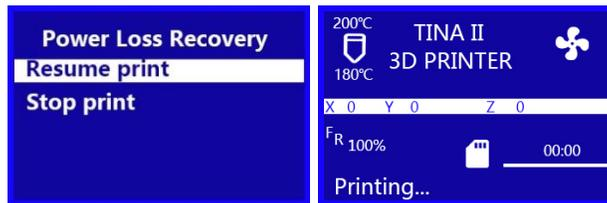
In the event that power is lost for any reason, the printer will remember where it was in the print process when power was lost. Perform the following steps to continue the interrupted print.
