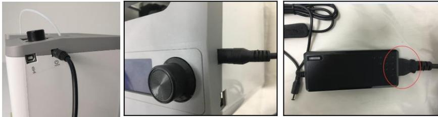
7. Flip the power switch on the inline control to the ON position (I). After the printer finishes booting, you will see the following wizard. Depress the Knob on top of the printer to select Next on the Welcome Screen, then again to select Next on the STEP 1: LOAD FILAMENT Screen.
