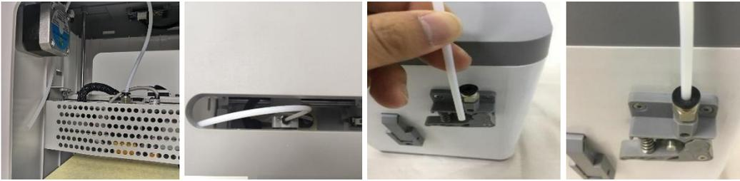
6. Ensure that the power switch on the inline control on the AC Power Adapter is in the OFF position (O). Plug the DC barrel connector on the AC Power Adapter into the Power Port on the right side of the printer. Plug the included AC Power Cord into the AC Power Adapter, then plug the other end into a nearby AC power outlet.
