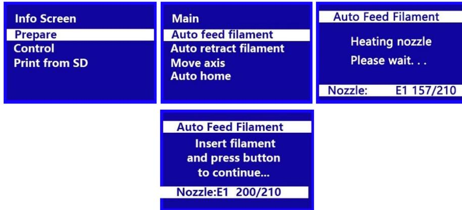
1. On the Main Menu, rotate the Knob until the Prepare option is highlighted, then press the Knob to enter the Prepare Menu.
