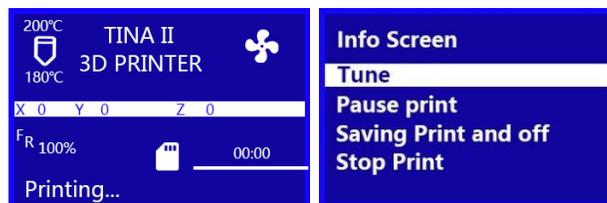
1. With the Printing... Screen displayed, press the Knob to display the Print Control Menu.
