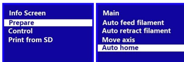
1. On the Main Menu, rotate the Knob until the Prepare option is highlighted, then press the Knob to enter the Prepare Menu.
