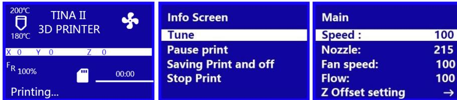
1. With the Printing... Screen displayed, press the Knob to display the Print Control Menu.
