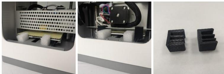
4. Rotate the Coupling Screw clockwise to lift the Magnetic Print Bed, then remove the foam block from under the print bed.
