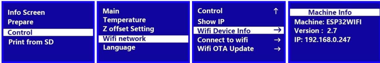
1. On the Main Menu, rotate the Knob until the Control option is highlighted, then press the Knob to enter the Control Menu.
