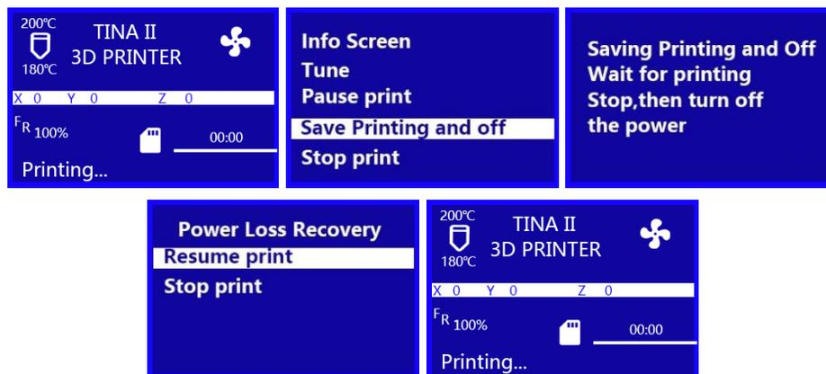
The Tina 2 printer features the ability saving a print in progress, so that you can turn the printer off and resume printing at a later time. Perform the following steps to save and resume a print in progress.
