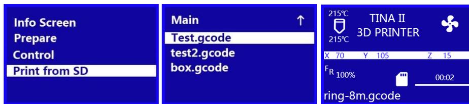
1. On the Main Menu, rotate the Knob until the Print From SD option is highlighted, then press the Knob to enter the File Selection screen.
