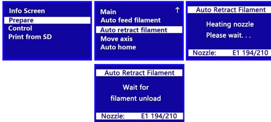
On the Main Menu, rotate the Knob until the Auto Retract Filament option is highlighted, then press the Knob. The Nozzle will heat to the target temperature. Once the target temperature is reached, the Extruder motor will retract the existing filament.
