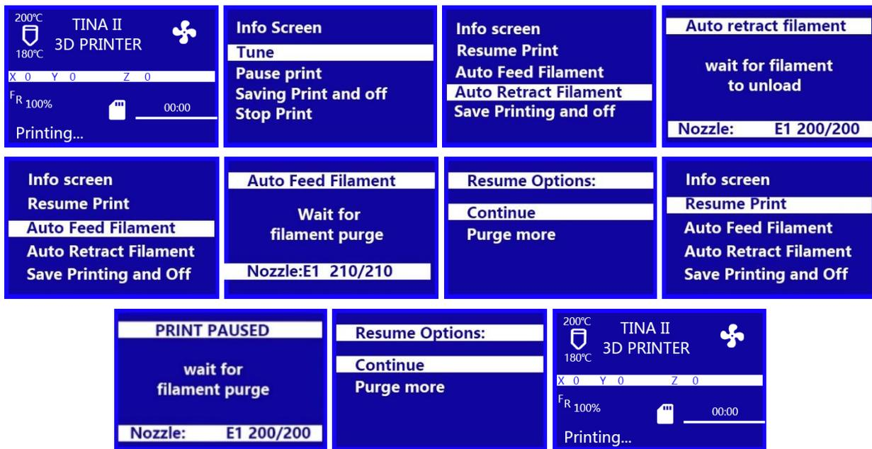
1. With the Printing... Screen displayed, press the Knob to display the Print Control Menu.
