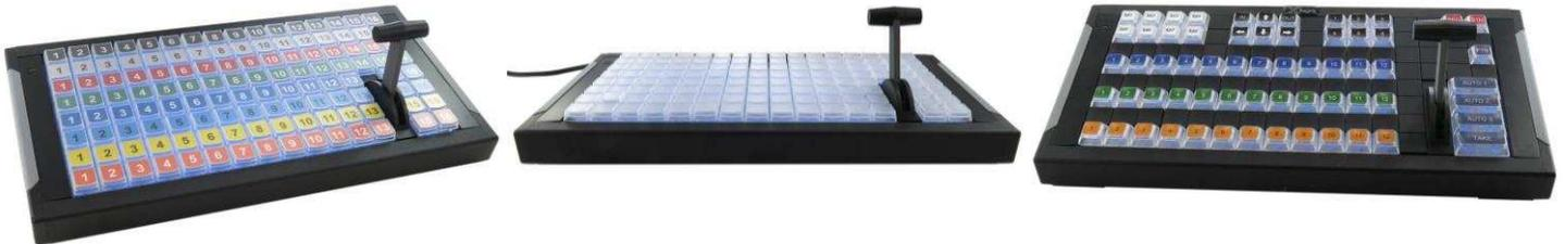
Our largest programmable controller, the XKE-124 T-bar offers one hundred and twenty-four keys plus an embedded T-bar in a commercial duty extruded aluminum case. Optional key blockers, and large keys instantly customize the XKE-124 to fit your requirements. Perfect for creating a cost-effective video switcher or for any system requiring linear input control.
