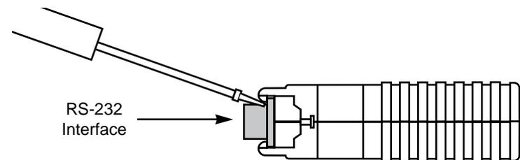
**Figure 1.** Inserting the screw driver
