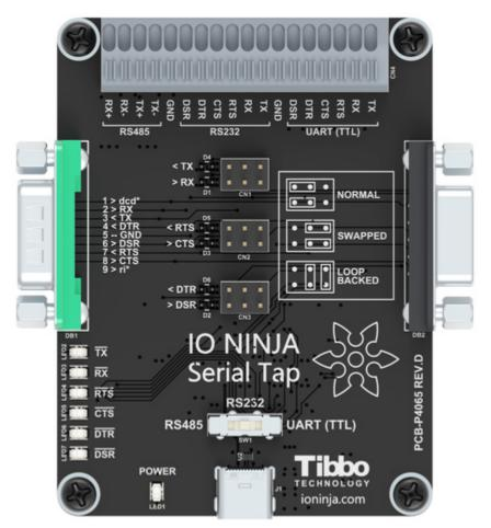
Serial Tap is an affordable serial sniffer that can monitor RS232, RS485, and TTLlevel UART communications. The Tap connects to your PC via a USB cable and is compatible with IO Ninja terminal/sniffer software.
