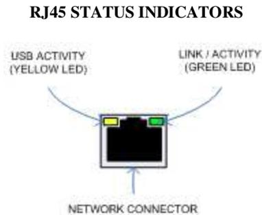
The USB Activity is a yellow indicator. The USB Activity is solid yellow when the LAVASynC+ is powered and connected to the device. The USB Activity flashes when there is traffic between the device and a LAVASynC+ product.
