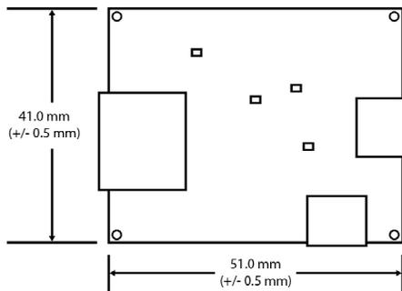
**Dimensions of the LAVASynC+ BM-OEM board**
