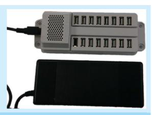
2) Insert the C13 connector from the power cord into the C14 receptacle on the power supply.
