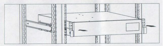
Step 5: Fix the UPS in position with 4 screws.
