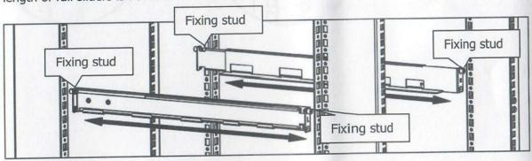
Step 2: Use 4 pieces of M6 screws to mount rail sliders into chassis. See chart below:
