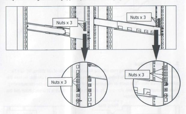
Step 4: Put UPS with assembled ears on the rail support.
