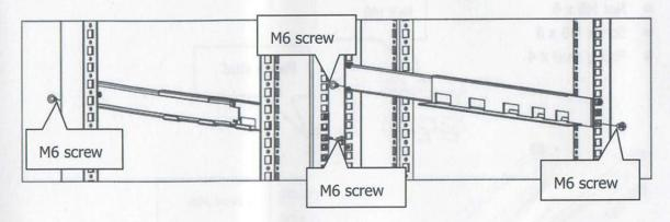
Step 3: According to UPS height, put 6 pieces of nuts on proper location.
